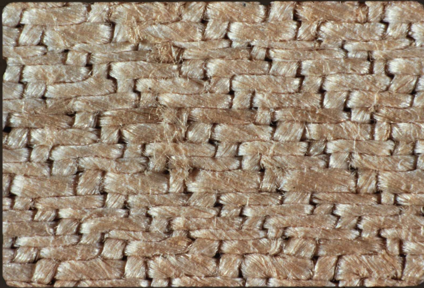
Herringbone weave, .3 mm thick
