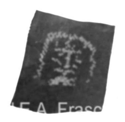
Shroud-like face imprinted by UV laser pulses. It is well visible when making the negative of the image. Even the single laser shots can be recognized.
