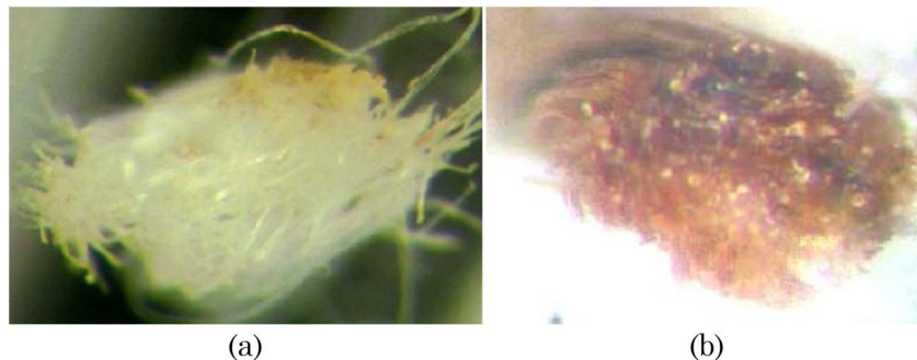
Fig. 6. (Color online) Photomicrographs of the cross section of two linen threads, irradiated by (a) ArF and (b) XeCl laser beams, respectively, “from top” of photos. In (a) VUV colors a very thin topmost part of the thread, corresponding to few fibers. In (b) UV colors more than one half of the section of the thread. Both threads have an average diameter of 300 \mu\text{m} [35].
