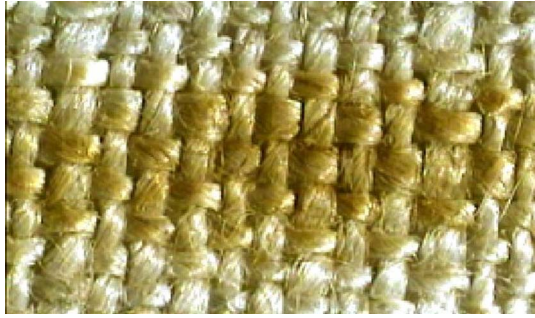
Fig. 3. (Color online) Photomicrograph of the cloth irradiated with 100 XeCl laser pulses. Intensity (fluence) = 16 MW/cm 2 (0.5 J/cm 2 ) per pulse.
