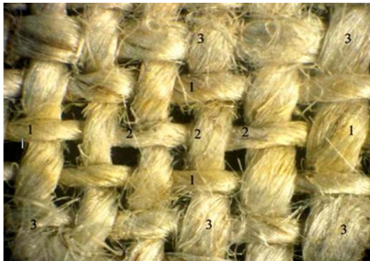
Fig. 5. (Color online) Area of the linen irradiated by the ArF laser beam shows different characteristics that depend on the local values of F(x,y) . (1) Colored area, (2) ablated area, and (3) area irradiated below the threshold for coloration [36].
